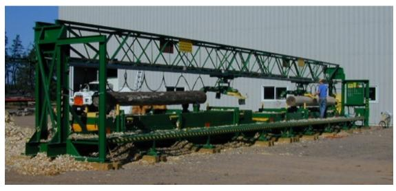
The largest of the long log peelers, this model allows the option of a log turning chuck over the standard driven turning rollers. Adjustable rollers support the log along its length. The cutting head is suspended from tracks that run the entire length of the frame, giving more flexibility and clearance in the working area. This model shown uses the option of a second cutting head, which allows two operators to work on the same log or on two shorter logs simultaneously.
